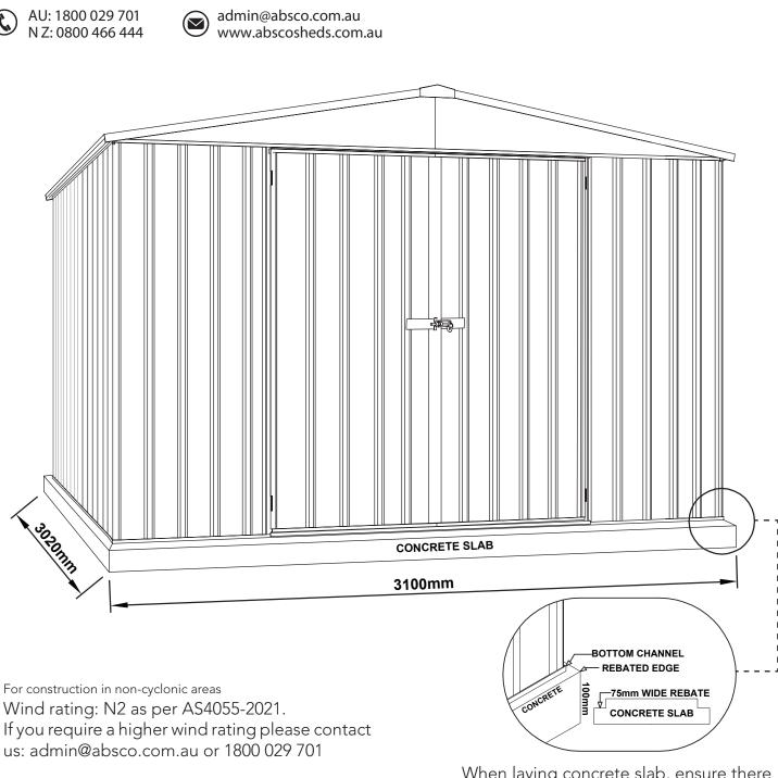
NOTE: This shed can be upgraded to wind rating: C1 as per AS4055-2021 with the additional purchase of a Cyclone Kit.
