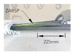
Step 2. Use the ZARSP to connect at the centre of the two ridge beams. Be sure it is pushed in fully.
