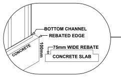
When laying concrete slab, ensure there is a rebated edge 25mm deep around the perimeter. This will help water egress from the base of the shed.
