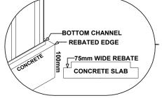
When laying concrete slab, ensure there is a rebated edge 25mm deep around the perimeter. This will help water egress from the base of the shed.
