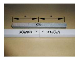
Step 1. Position the channels and the CSJ joiner so the centre of the CSJ is in line with the end of each channel to be joiner together.
