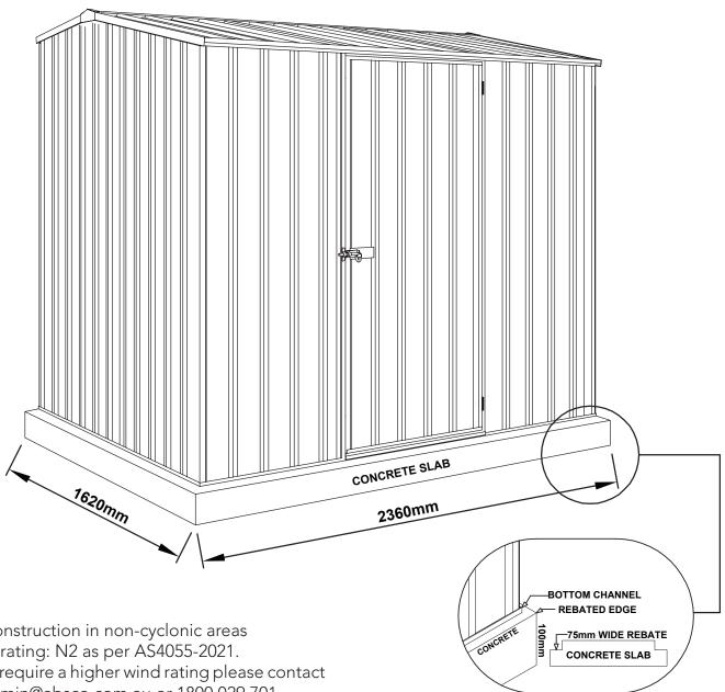
For construction in non-cyclonic areas Wind rating: N2 as per AS4055-2021. If you require a higher wind rating please contact us: admin@absco.com.au or 1800 029 701
