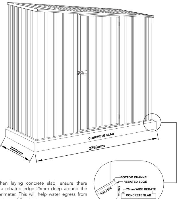
When laying concrete slab, ensure there is a rebated edge 25mm deep around the perimeter. This will help water egress from the base of the shed.
