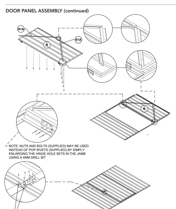
NOTE: The two holes required to connect the padbolt hasp for each door have not been pre-punched, to allow for proper alignment. position each hasp centrally over the padbolt shaft, and drill 3mm holes and secure with screws
