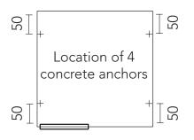
Each anchor consists of one nut, bolt, dynabolt and steel angle.
