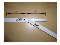
Step 3. Join the second channel to the CSJ by positioning the << JOIN of the channel at the centre of the CSJ, on an angle. Push the CSJ into the channel until you hear a 'click'.
