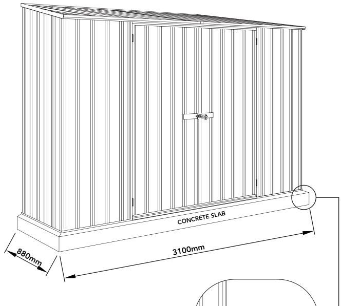
When laying concrete slab, ensure there is a rebated edge 25mm deep around the perimeter. This will help water egress from the base of the shed.
