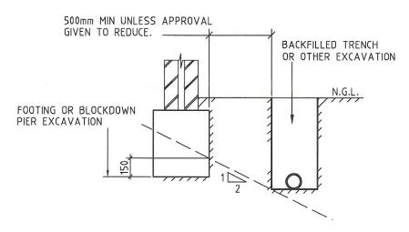
The contactor shall undertake investigatory localised excavations near footings to ascertain their depth prior to excavating adjacent to them. It is noted that excavating to a depth below that indicated above shall not be undertaken without the written approval from the engineer.
