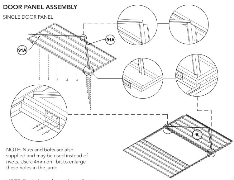
NOTE: The holes to fasten the padbolt hasp are not pre-punched to allow for proper alignment. Position the hasp centrally over the padbolt shaft and drill 3mm holes and secure with screws.
